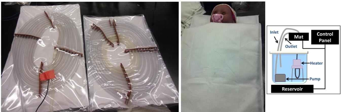
Figure 2: Our R&D team is hard at work testing and refining our designs to find the most appropriate solution for the developing world. Left – Picture of the design which uses a warm water circulation system made of biocompatible materials such as PVC tubing and plastic to provide heat to the infant. Middle – Prototype, including fold-over component, in use. Right – System diagram.
